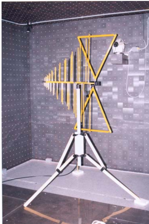
EN 61000-4-3 Radiated Radio Frequency Ferrite Tiled 12' x 20' x 10' Chamber with Uniform Field at 3 & 10 volts per meter
